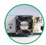
Hot-plug fans: 2 minutes maintenance time, no need to open or switch off the unit.
