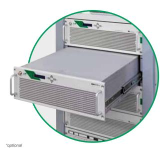
The above PFG Series transmitters are available also as amplifiers, without the internal exciters, with the name of KFG Series
