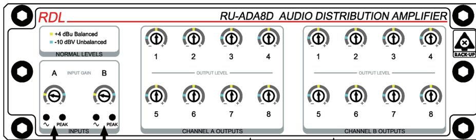
WITH NORMAL INPUT SIGNAL CONNECTED, TRIM INPUT GAINS FOR CORRECT LEVEL ON DUAL-LED METERS (GREEN LED BRIGHT AND RED FLASHING OCCASIONALLY)
