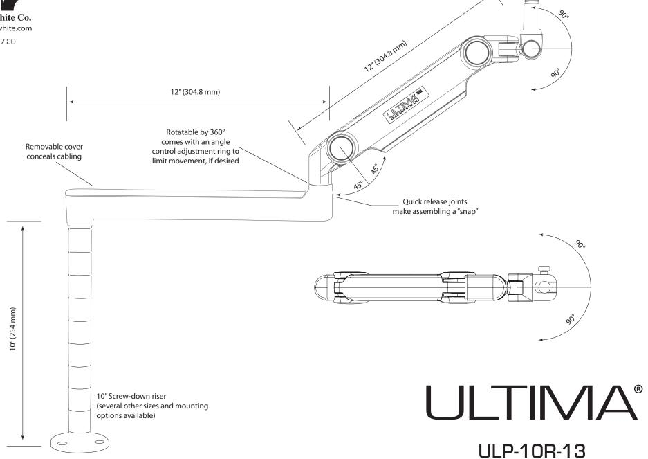
Ultra Low Profile Mic Arm with 10" Riser Aluminum construction • Black finish
