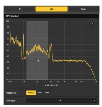
L-R component in this case. The value posted below the plot is the same as that indicated on the Meters menu.
