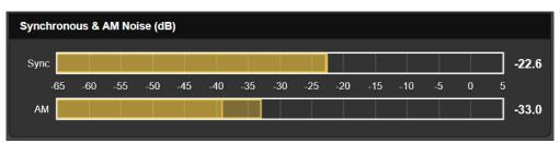
Sync (synchronous) FM noise refers to amplitude modulation of the FM carrier by the FM baseband signal, predominantly by program audio. If the passband of the transmitter is not frequency-flat, then as the carrier deviates toward the channel frequency extremes the carrier level might undergo amplitude rolloff at the band edges, which would amplitude-modulate the FM carrier.
