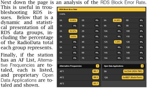
Clicking the Clear/Reset RDS bar at the bottom will indeed clear the registers and begin a new RDS data collection. Reset is automatic when the station is changed.
