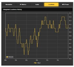
the Time Span: to cover a longer sampling period, vertical scaling will change to accommodate the level range for that particular timeframe.
