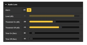
In this case we're looking for a low-level program audio condition, so the Threshold On (dB): setting of –20 is what the program level has to fall to, and remain below, for the Time On (Sec.) interval of 10 seconds to initiate an alarm.
