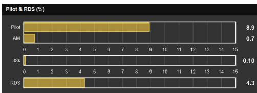
This next section of the display screen first shows the injection level of the 19kHz stereo pilot. On an FM station broadcasting in stereo, Pilot should be a rock-steady reading of about 9.0%. Composite clipping or other nonlinearity in the transmission path can cause this reading to 'bounce' to a lesser or greater extent. These level perturbations will show up on the accompanying AM bargraph as amplitude modulation of the stereo pilot.
