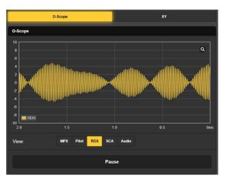
Pause bar at the bottom of the screen lets you freeze the waveform. The little magnifying glass in the upper-right corner will switch you to a full-screen display.
