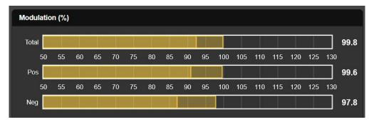
These three bargraphs and their associated numerical readouts on the right give quasi-peak-response measurement of FM carrier deviation. Total modulation and individual Pos and Neg deviation are shown in percent, 100% equal to ±75kHz deviation.
