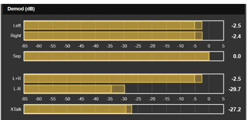
This metering area displays the demodulated FM program audio. Left and Right channel levels have quasi-peak response and a rapid fallback to give a good visualization of instantaneous vs. average program energy. Bear in mind that these meters in no way approximate true "VU" ballistics. A floating peak-hold 'ghost' hovers briefly above these meters showing the highest peak value recently indicated. This held value is also shown numerically at the right of the bargraph.
