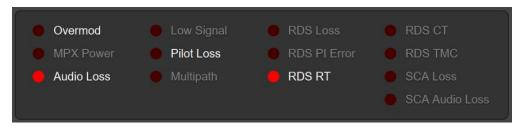
This Now Playing alarm panel is a duplicate of the one on the Alarms Webpage. Setup of the alarms and alarm messaging is detailed in that discussion section.
