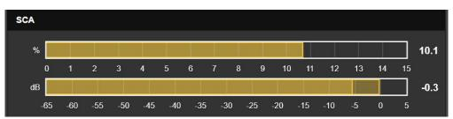
The % scale shows the injection level of the SCA subcarrier in percent of total FM carrier modulation. The traditional figure of 10% indicates ±7.5kHz deviation of the carrier. The dB scale displays the audio level of the recovered SCA program. 0dB equates to the deviation set by the Now Playing / Tuner / SCA / Deviation (kHz): slider (Page 19.) With the slider at its default of 5.0, ±5kHz SCA deviation by a steady-state tone would drive dB to 0.
