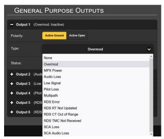
The alarm function assigned to each tally line is listed, and you can specify alarm tally Polarity:, whether you want an Active Ground (chassis ground) or Active Open (open circuit) when the alarm is triggered.
