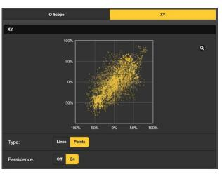
When XY is implemented with a traditional analog oscilloscope, the display resembles a 'connect-the-dots' image of the so-named children's activity. The 541 and most digital 'scopes can optionally show either Lines or Points. The Points option presents a more artistic 'constellation' as seen in the example, and in this instance Points and Persistence were both engaged to show the short-term trend of the stereo image.
