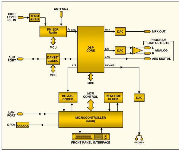
Block Diagram of the Inovonics 541 FM Modulation Monitor
