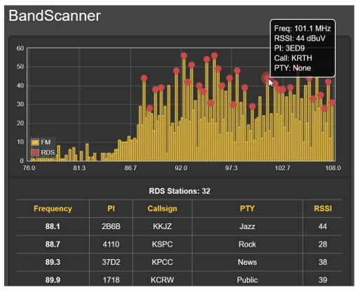
Shown above is an entire FM-band plot of the busy Los Angeles FM market. Two Scan Type: modes may be selected at the bottom of the screen. RSSI is the quickest scan, but will show only RSSI signal levels. But the 541 can also scan and display both RSSI + RDS information, which will take a bit longer.
