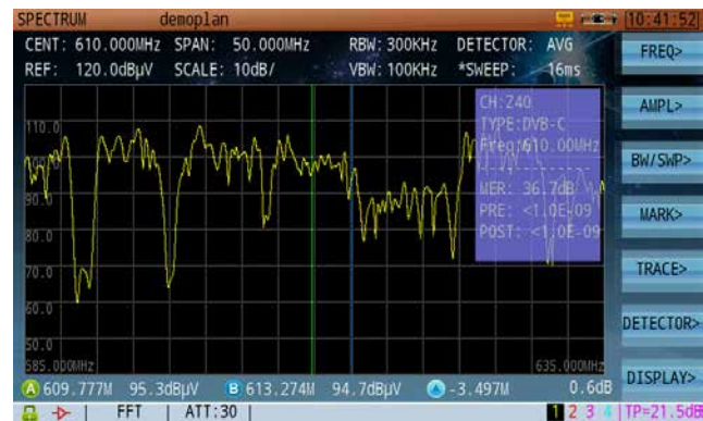
Figure 5: Simultaneous Display of Spectrum and QAM Analysis
