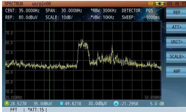
Figure 6: Spectrum Analysis: Low Level Signal Covered by High Level Signal
