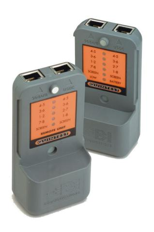
Low Cost Structured Cabling "Wire Map" Tester
