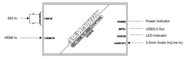
Note: When both SDI and HDMI are plugged, SDI input signal will take priority. When both SDI/ HDMI IN and AUDIO IN are plugged, exteral audio input will take priority.
