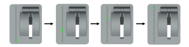
3) Adjust the T-Bar to A-BUS or B-BUS until all LED indicators turn on. Below image is an example of the LED indicators status when switching the T-Bar from B-BUS to A-BUS.
