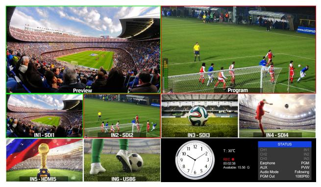
2) The following 6 windows come from the 6 input signals. The signal source of window 5 and 6 can be selected from HDMI, DVI, VGA, USB.
