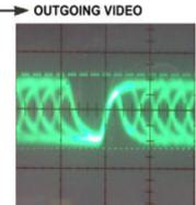
induced noise affects the absolute bit timing it can result in lost data. Looking at an eye pattern for HD-SDI affected by extraneous induced noise (**Incoming Video**) the data zero crossing point (risetime/falltime area) appears smeared indicating the potential for a bit error and the loss of data. Using
