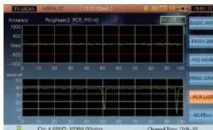
PCR Interval and PCR Accuracy Monitoring
