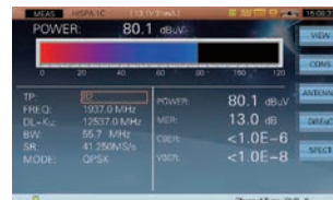
DVB-S/S2 Signal Measurement
