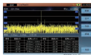
DVB-T2 Echo pattern displaying to locate the SFN interference
