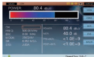
QAM signal quality measurement
